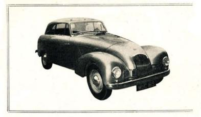
The ALLARD Saloon, with aluminium-panelled coachbuilt body, incorporates the good features of all the other models, including sports-car manners on the road, plus such refinements as steering column gear-change and independently-adjustable close-fitting front seats allowing ample room for three abreast, luxurious hide upholstery with Latex cushion rubber, interior lighting with door-operated switch, heating and demisting equipment and controlled air conditioning.
