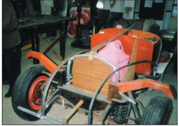
Steel skeleton in place, note cardboard templates
