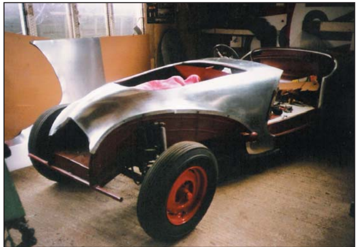
Fenders removed with hood in place
