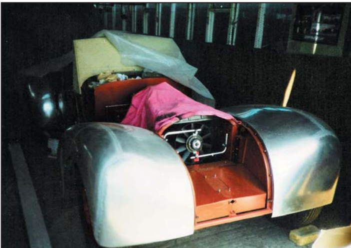
Front fenders installed without headlight ports cut
