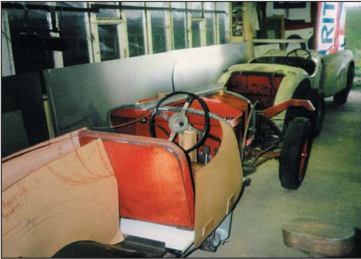
Cardboard templates in place, note reference K2 in the background
