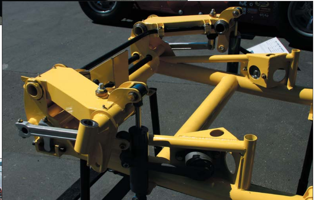
The surprisingly → complex front suspension of a “crude” Indy roadster.
