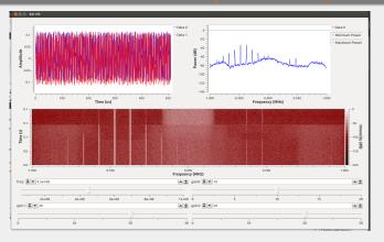
• Increased power completely distorts the received signal.
