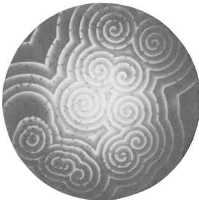
Figure 6. The Belousov-Zhabotinsky chemical reagent, seen by blue light transmitted through a 1 mm depth. The bright spirals mark loci of maximum concentration of ferriin (Belousov's blue indicator dye); the intervening darkness is deep orange. Waves of oxidation propagate from the spiral centers at a few mm per minute, the spirals turning in about one minute. The dish is 90 mm in diameter. From Winfree and Strogatz [29], Figure 2. (This figure originally appeared in an article by A. T. Winfree and S. H. Strogatz, Physica-8D (1983), pp. 35-49, North-Holland Physics Publishing, Amsterdam.)
