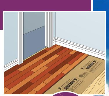
Aquabar "B" floor and tile underlayment is an extremely effective moisture vapor retarder for use in a variety of interior construction applications. Consisting of two layers of kraft paper laminated with asphalt, Aquabar "B" is a non-reinforced 30/30/30 duplex type Grade "B" paper.
