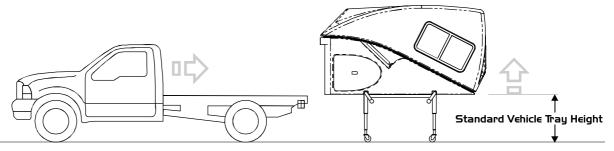
Once the host vehicle is positioned under the slide-on the jacks can be lowered until the weight of the Innovan is carried by the vehicle. The jacks can then be removed and stored. Before you start your adventure, make sure that the slide-on has been fastened to the trayback using supplied Innovan mount brackets. Also connect any power supplies your slide-on may require from the host vehicle.
