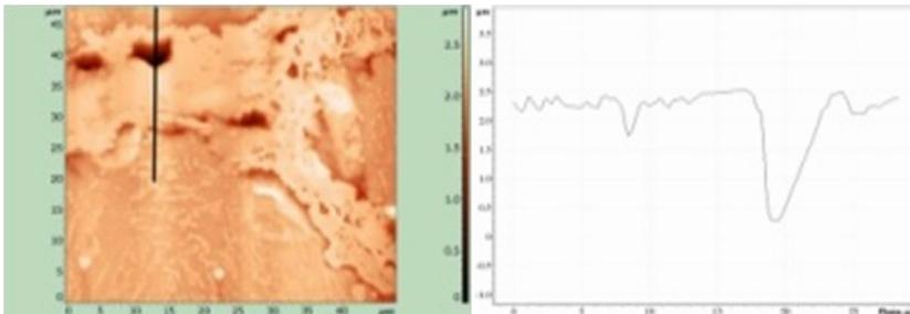
SFM image acquired after chemical etching of a P91 sample. The cross-section along the black line is on the right, highlighting the cavity in the image.
