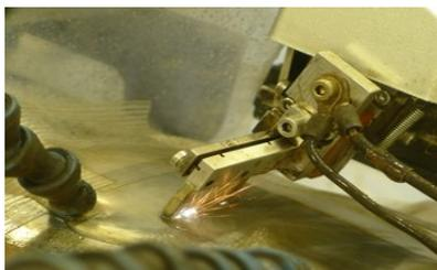
On the left, is a picture of the EDSE cutting out a small slice of a pipe and on the right is a picture of the SFM detecting for any creep damage.
