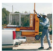
All UL models are fitted with the EZ loader system to assist loading onto pickup trucks.
