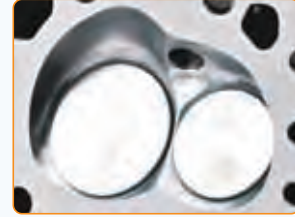
CNC-Profiled Combustion Chamber (54cc combustion chamber heads only)
