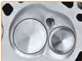
CNC-Profiled Combustion Chamber
