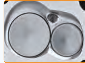
CNC-Profiled Combustion Chamber
