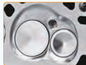
CNC-Profiled Combustion Chamber
