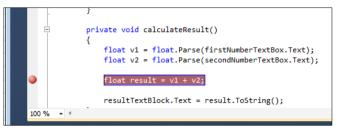
The line is highlighted as shown above. You can clear a breakpoint by repeating the process. When the program reaches the breakpoint it will stop running and you will be able to take a look at the values of the variables.
