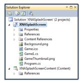
The file GameThumbnail.png holds the image to be used in the application list. The file Background.png holds the image to be used when the application has been "pinned" to the Start menu.
