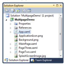
We can regard App.xaml as the container for the phone application. It provides the context in which the pages are displayed. It doesn't actually ever get drawn on the screen, but it is the starting point for the application when it is loaded. The App.xaml.cs file contains the methods that start an application running. It also contains handler methods for application lifecycle events which we will be using later.
