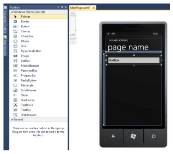
Above shows the effect of dragging a TextBox out of the Toolbox area and dropping it onto the Windows Phone page. If we run the program now we can see our textbox on the screen:
