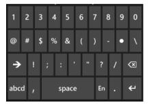
It would be nice if each TextBox in the adding machine could be set for numeric entry when that TextBox is opened. We could do this by modifying the properties of the TextBox when the program starts running but the best place to put such settings is in the XAML description of the control itself. At the moment the XAML that describes the secondNumberTextBox is as follows:
