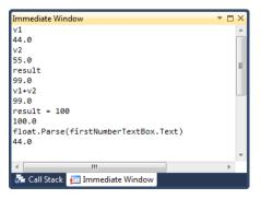
If I just type the name of a variable the window displays the value in that variable. I can also type in expressions (e.g. v1+v2 as shown above) and these are evaluated and displayed. I can also assign a value (e.g. result = 100) and call methods on objects to work out results.
