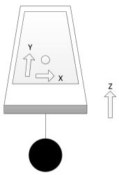
If we hold the phone flat as shown, the weight will hang straight down underneath the phone. If we were to measure the distance in the X, Y and Z directions of the weight relative to the point where it is attached to the phone it would read 0, 0, -1, assuming that the spring is length 1. The value of Z is -1 because at the moment the position of the weight is below the phone and the coordinate system being used has Z, the third dimension, increasing as we move up from the display.
