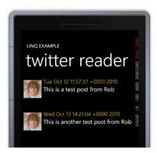
This is very nice. It means that you can display any collection of data in a list on the page just by setting them as the source for a ListBox. All you have to do is create a data template that binds the properties of each instance to display elements and then assign a list of these instances to the ItemSource property of the ListBox.
