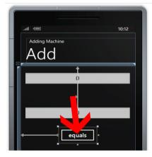
The picture above shows where we should double click in Visual Studio. When we double click on the button Visual Studio sets the properties of the button in XAML to connect the button to a method in our page. It also creates an empty version of that method and takes us straight to this method, so that we can start adding the code that must run when the button is clicked.
