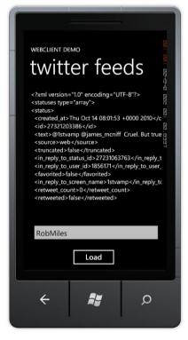
This makes it very easy to make a slightly modified version of our WebClient program that assembles a web request for the Twitter server and uses that to read feed information from it. The only change we have to make is to the code that produces the web request:
