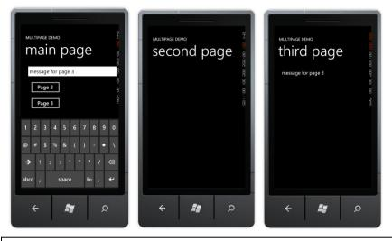
The solution in *Demo 08 Multipage Demo* is a three page Silverlight application. You can move to pages 2 and 3 by pressing buttons on the main page. You can return from Page 2 by pressing the back button. If you use the back button on page 3 you need to respond to a confirmation dialog before being moved off the page. Text entered on the main page is transferred into a TextBlock in page 3 via the page uri.
