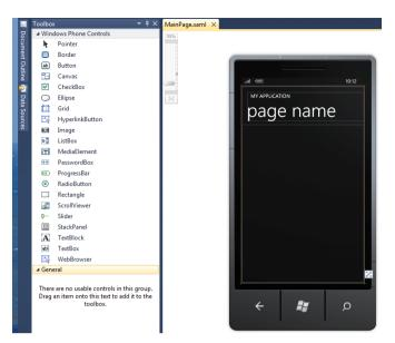
We can assemble the user interface by simply dragging the controls out of the toolbox onto the design surface.
