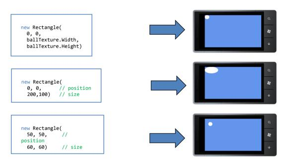
The first version of our program drew the ball with the same size as the original texture file. However, we can use whatever size and position we like for the drawing process and XNA will scale and move the drawing appropriately, as you can see above.
