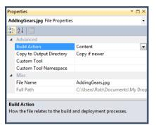
Content assets are copied by Visual Studio into the application directory when the program is built. The "Copy if newer" setting means that Visual Studio will copy a new version of the image into the binary folder if the current image in the project is replaced by a newer file.
