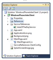
Once the service has been added it now takes its place in the solution. Our application must now create a proxy object that will be used to invoke the methods in the service. The best place to do this is in the constructor of the main page:
