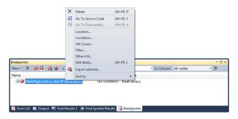
You can use this window to set breakpoint properties. You can request that a breakpoint only fire after a given number of hits, or only fire when a particular condition fires. This is terribly useful. You might have a program that fails after the fiftieth time round a loop. It is very nice to be able to add a counter or a test so that the program skips past the breakpoints you are not interested in.
