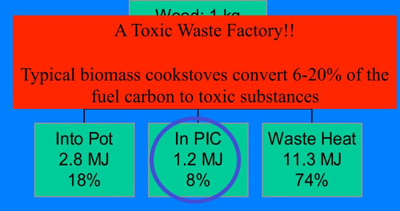
PIC = products of incomplete combustion = CO, HC, C, etc.
