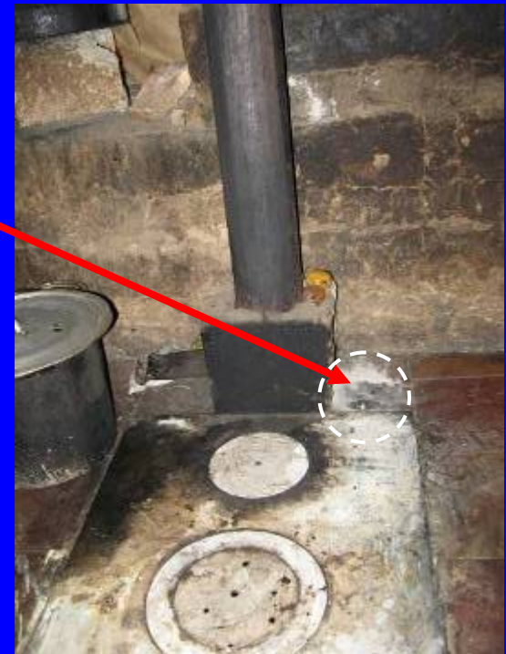
Monitoring drop out rates and patterns of use with the SUMS system
