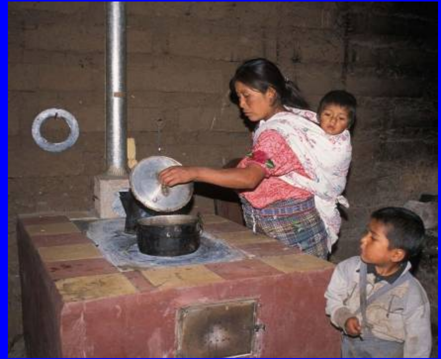
Chimney wood stove, the Plancha, locally made and popular with households
