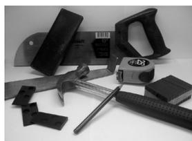
When sawing pieces off the planks, use a fine-toothed hand saw, jigsaw or cross-cut saw.
