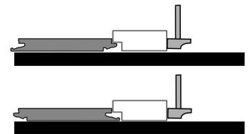
edge, use several small taps until the planks click together completely. For a long edge, tap planks together gradually. Begin tapping lightly at the corner of a plank until the joint has clicked together. Repeat the process approximately every 12" (30cm) until the entire long edge of the plank has clicked in with the next plank. Never attempt to knock the Uniclic® joint into place with just one hit.
