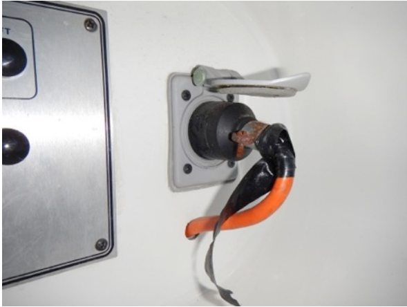
120V AC power outlet is not ignition protected
