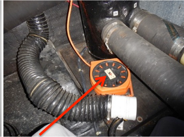
120V AC power outlet is not ignition protected
