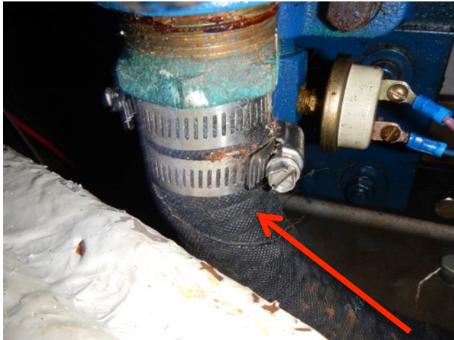
Main engine raw water intake hoses appear in questionable condition
