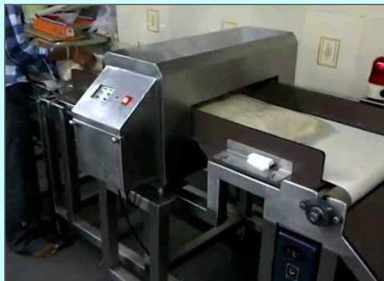
exception is if the processor writes metal detector use into the HACCP plan. If it appears in the HACCP plan, it must be utilized. We in the food safety arena can attest that metal detectors are absolutely needed for every firm who processes food through metal equipment. Unfortunately, due to their high cost and the fact that they are not part of the manufacturing process they are often not included.
