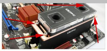
2. Attach the waterblock to the top of the side plates by using the silver screws and allen key.
