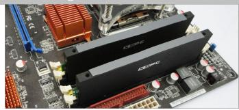
1. Fit the memory modules and place thermal pads on the top of each heat spreader.
