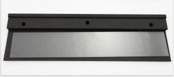
2. Remove the tape from both sides of a thermal pad and place it on the position shown above. You may have to trim the thermal pad to size.
