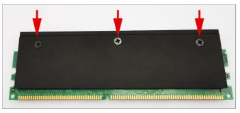
5. Place the back of the side plate over the memory module and carefully tighten the 3 screws shown above.
