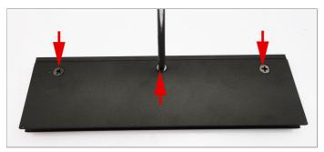
1. Unscrew the 3 screws from the back of the memory side plate.
