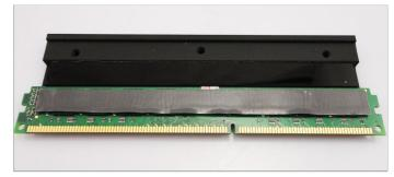
**6**. Remove the tape from both sides of the second thermal pad and place it over the memory module.
