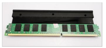
5. Place the memory onto the thermal pad and make sure it is positioned in the centre of the side plate.
