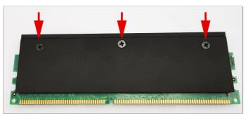
7. Place the back of the side plates over the memory module and carefully tighten the 3 screws shown above.
