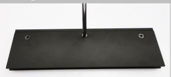
1. Unscrew the 3 screws from the back of the memory side plates.
