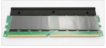
**4**. Remove the tape from both sides of the second thermal pad and place it over the memory module.
