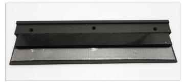
**4.** Remove the tape from both sides of a thermal pad and place it on the position shown above. You will have to trim the thermal pad to size.
