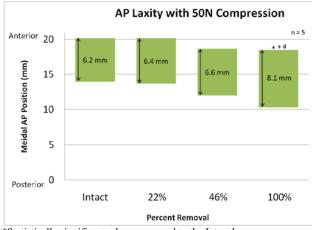
\*Statistically significant when compared to the Intact knee +Statistically significant when compared to the knee after 22% resection #Statistically significant when compared to the knee after 46% resection **Graph 1**: At 50N of compression, increasing the amount of medial meniscus resection leads to increased posterior translation of the medial femoral condyle.
