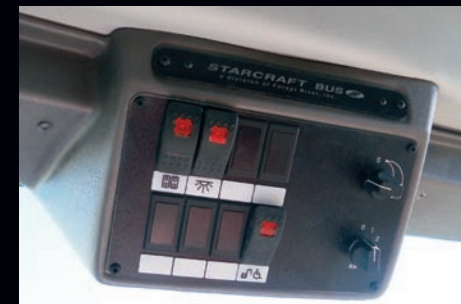
Driver's switch panel conveniently located within view of the road and not on the engine cover
