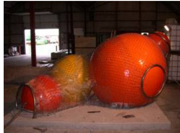
Img. 7: Inflatable mould; Butink-technology.com (2011)
