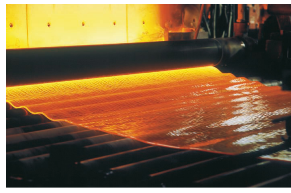
Img. 5: Heated glass taking shape by its own weight; [4] (2011).
