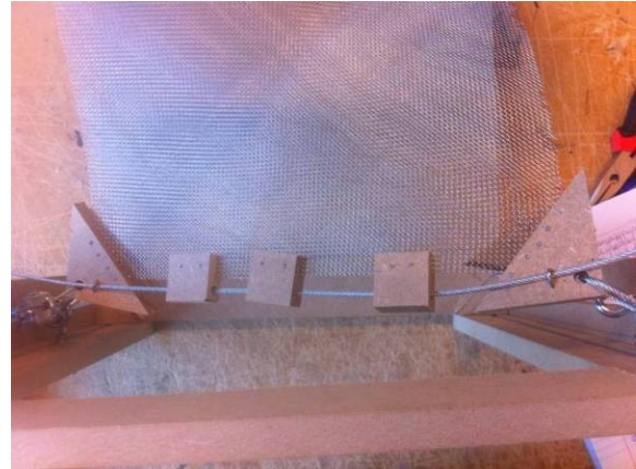
Img. 20: Edge tensioning with clamps connected to an edge cable
