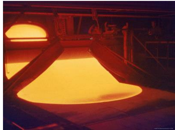
Img. 4: Heated glass with low viscosity; saddoboxing.com (2011)
