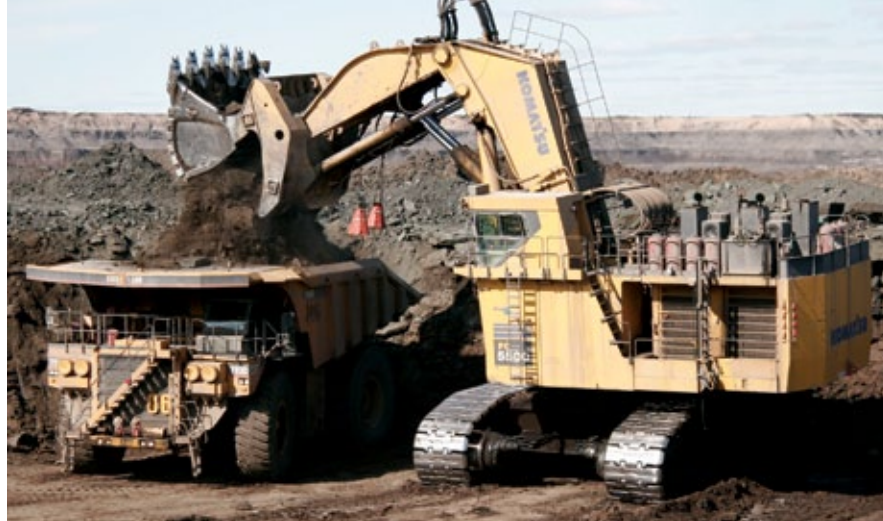
KMC Mining PC5500 loading overburden in to a Cat 793 at an oil sands site. (Photo courtesy of KMC Mining).
