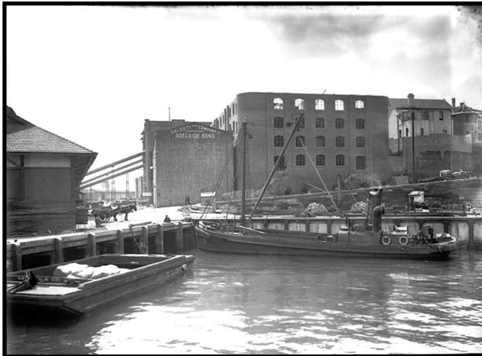
Figure 33. "A steam lighter at the Munn St wharf, Millers Point (NSW)," c. 1 January 1941 (Photo: State Records of New South Wales).
