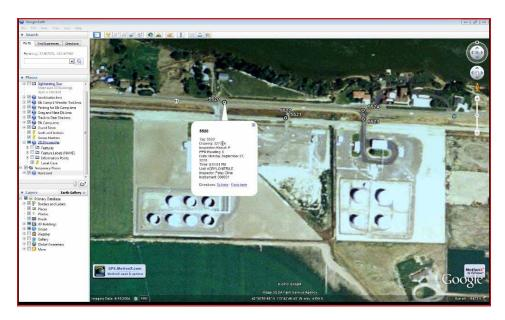
So here's the monitoring that Patsy did. We'd see the tank. She was right at the entranceways to the tank farm here. The individual tags that she monitored are the points. If I click on any of those points, it opens up and gives me the details. Here's the tag, the drawing, the inspection, the date she did the inspection, the unit she was in and so forth. If she had found any leaks, the leaks, instead of being black, the leaks would show up as red.
