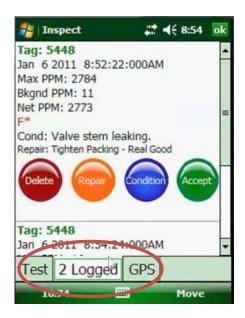
And at this point, now, notice very closely. I have two log readings on my tab and I can see both of those log readings just by scrolling down. So the first reading at 8:52 was 2700 PPM. The condition was that the valve stem was leaking. The repair was made. They tightened the packing real good. And then I did a retest at 8:54. Got a reading of 16 PPM. Once I'm good with this, I'm just going to hit the accept button.
