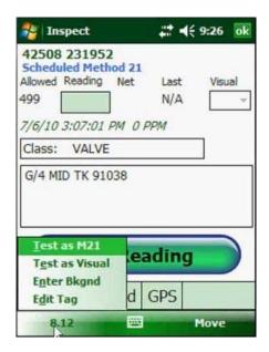
I can force the test type to change from a Method 21 to a visual or from a visual to a Method 21. I can force a test type change. I can enter a background reading, just like I did previously, or very importantly, I can edit the tag. And that's what I want to show you here is my technician had a hard time finding this component. I'm going to click on the edit tag button. That takes me into edit mode on this component.
