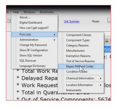
Chemical information has its own little sub-menu – chemical names, stream names, batch names, also a mobile calibration gas that gets downloaded out to LeakDAS mobile – location information – those five location fields – and then your instrument list where you can build your list of the different TVAs or OVAs or whatever you're using in your facility.
