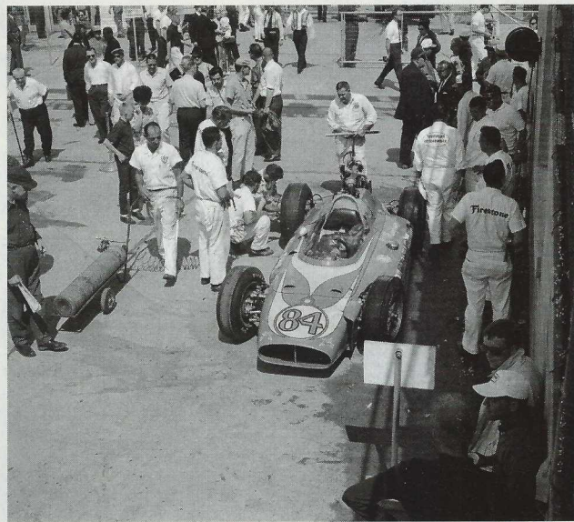
> In 1962 Thompson went after the holy grail of American motorsports, the Indy 500. Beating Colin Chapman by a year, he shocked Gasoline Alley with three mid-engined cars powered by Buick aluminum V-8s. Dan Gurney, a rookie at Indy in 1962, finished Eighth driving one of the Thompson specials.
