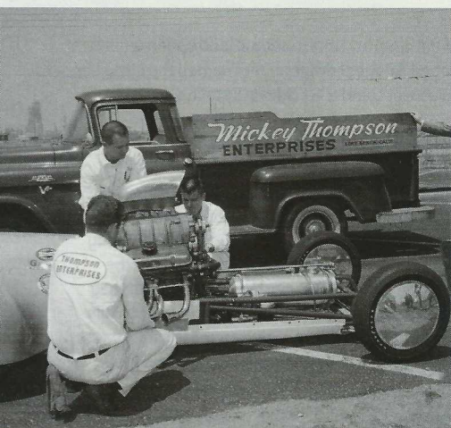
> Mickey's streamlined dragster, Assault, in May 1960. The blower setup he and Fritz Voigt devised for Assault's Pontiac V-8 helped them science out the four GMC superchargers on Challenger I.
